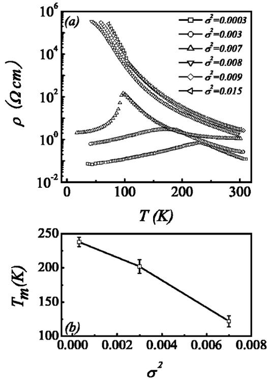
FIG. 2. (a) Zero-field resistivity  $\rho$  as a function of  $T$  for all the samples with  $\sigma^2$  from 0.0003 to 0.015. (b) Measured dependence of  $T_m$  on  $\sigma^2$ . The unit of  $\sigma^2$  is  $\text{\AA}^2$ .
