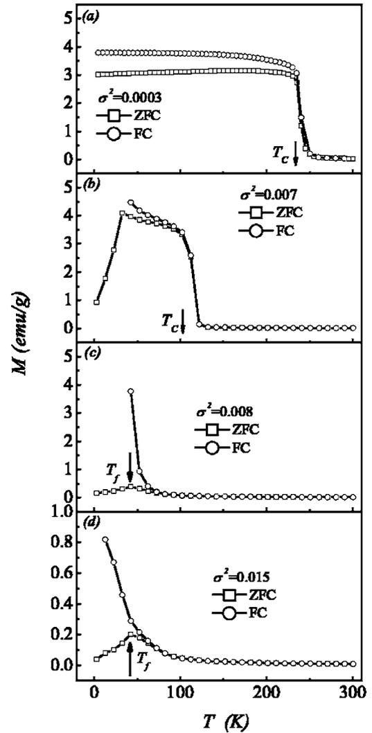
FIG. 3. Measured magnetization  $M$  as a function of  $T$  measured during warm cycle for samples of (a)  $\sigma^2=0.0003$ ; (b) 0.007; (c) 0.008; (d) 0.015; respectively, under the ZFC and FC conditions. The unit of  $\sigma^2$  is  $\text{\AA}^2$ .
