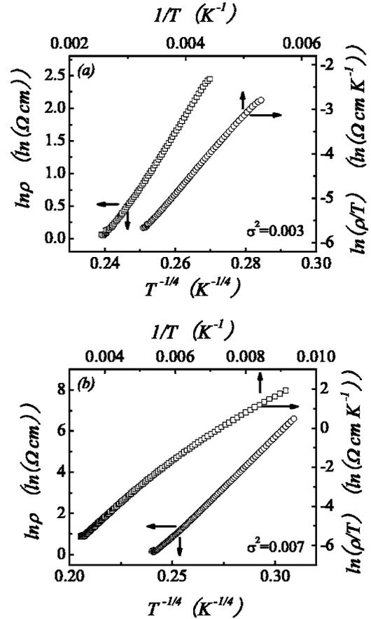
FIG. 7. Fitting of zero-field resistivity  $\rho$  as a function of  $T$  using the VRH model and small-polaron model for samples with (a)  $\sigma^2 = 0.003$  and (b)  $0.007$ . The unit of  $\sigma^2$  is  $\text{\AA}^2$ .
