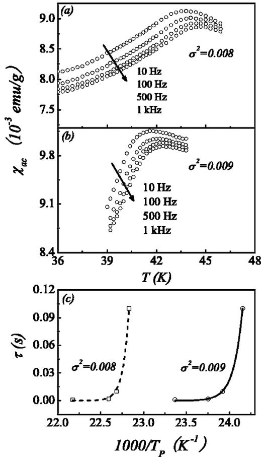
FIG. 6. Measured ac susceptibility  $\chi_{ac}$  as a function of  $T$  at four frequencies (10, 100, 500, and 1000 Hz) for samples of (a)  $\sigma^2 = 0.008$  and that of (b)  $\sigma^2 = 0.009$ , respectively. (c) Evaluated relaxation time  $\tau$  as a function of  $T_p$  (open dot) and fitting curves (lines) using the Néel-Arrhenius law. The unit of  $\sigma^2$  is  $\text{\AA}^2$ .
