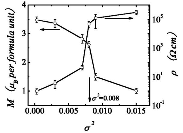
FIG. 5.  $\sigma^2$  dependences of magnetization  $M$  measured at  $T = 3$  K under a field  $H = 3$  T, and zero-field resistivity  $\rho$  measured at  $T = 50$  K. The unit of  $\sigma^2$  is  $\text{\AA}^2$ .
