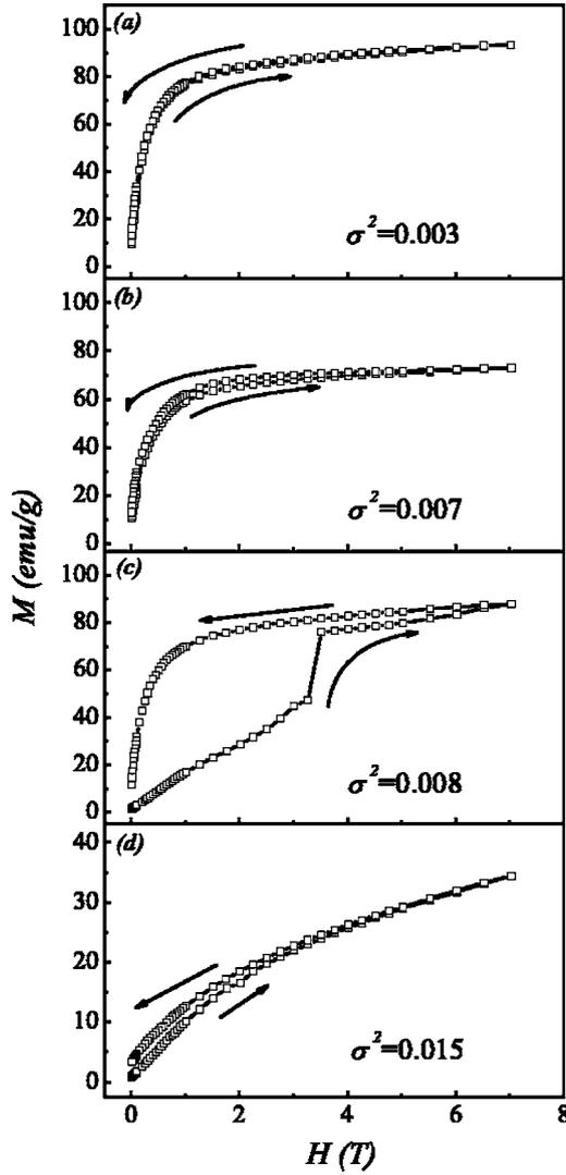
FIG. 4. Measured magnetization  $M$  as a function of  $H$  at  $T = 3$  K for samples of (a)  $\sigma^2 = 0.003$ ; (b) 0.007; (c) 0.008; and (d) 0.015, respectively. The arrows indicate the cycle of  $H$  varying during measurements. The unit of  $\sigma^2$  is  $\text{\AA}^2$ .
