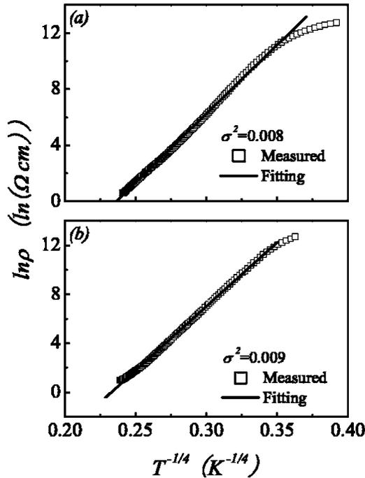
FIG. 8. Fitting of zero-field resistivity  $\rho$  as a function of  $T$  using the VRH model for samples with (a)  $\sigma^2=0.008$  and (b)  $0.009$ . The unit of  $\sigma^2$  is  $\text{\AA}^2$ .
