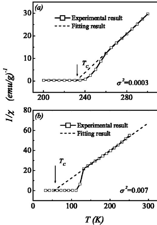
FIG. 10. Inverse susceptibility  $1/\chi$  as a function of  $T$  for the samples with (a)  $\sigma^2=0.0003$  and (b)  $\sigma^2=0.007$  measured under  $H=100$  Oe. The dashed lines are the fitting results following the Curie-Weiss law. The unit of  $\sigma^2$  is  $\text{\AA}^2$ .
