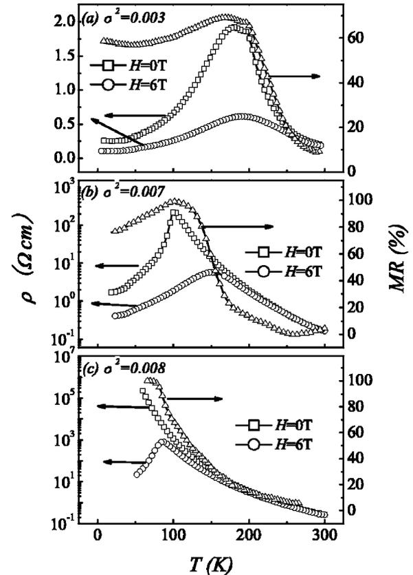
FIG. 9. Measured  $\rho(H=0)$  and  $\rho(H=6$  T) as a function of  $T$  for samples of (a)  $\sigma^2=0.003$ ; (b)  $\sigma^2=0.007$ ; and (c)  $\sigma^2=0.008$ , respectively. The MR ratio for each sample is plotted in the same figure. The unit of  $\sigma^2$  is  $\text{\AA}^2$ .
