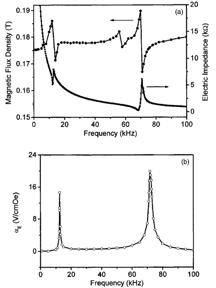
FIG. 3. (a) Frequency response of magnetic flux density for TEC piece and electric impedance for the PZT piece in the bilayer. (b) Frequency dependence of  $\alpha_E$  for the bilayer. An optimal  $H_{\text{Bias}} = 0.7$  kOe was set for maximum ME output.
