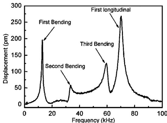
FIG. 2. Frequency response of the surface displacement of one free side of the bilayer induced by an ac magnetic field of 5 Oe at  $H_{\text{Bias}} = 0.7$  kOe.
