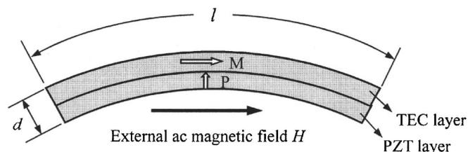
FIG. 1. Configuration and operation principle of the bending vibrational magnetoelectric TEC/PZT bilayer. The arrows  $P$  and  $M$  show the polarized direction of PZT and the magnetized direction of TEC, respectively.
