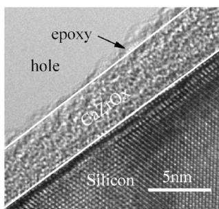
FIG. 2. Cross-section HRTEM images of the CZO-N films after the RTA processing. The film remains amorphous with a clean CaZrO<sub>x</sub>/Si interface.
