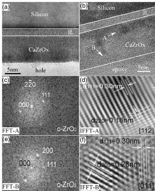
FIG. 1. Cross-section HRTEM images of the CZO-O films (a) before and (b) after the RTA processing. (c)–(f) are the FFT and IFFT images of the selected nanocrystals indicated by arrows A and B in (b), respectively.
