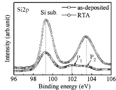
FIG. 3. Si2p core-level XPS spectra for the  $\sim 3$  nm thick CZO-O film before (as deposited) and after the RTA processing.
