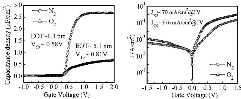
FIG. 5. (a) Capacitance density ( $C_{acc}/A$ ) and (b) leakage current density ( $J$ ) as a function of voltage ( $V$ ) for Pt/CaZrO<sub>x</sub>/n-Si capacitors with the CZO-N and CZO-O films, respectively. Both the films are  $\sim 3$  nm thick and undertaken the RTA processing.
