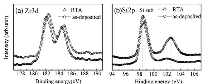
FIG. 4. XPS spectra of (a) Zr3d and (b) Si2p core levels for the  $\sim 3$  nm thick CZO-N film before (as deposited) and after the RTA processing.
