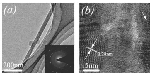
FIG. 2. (a) TEM image of an isolated BFO nanowire with the SAED pattern in the inset; (b) high-resolution TEM image of the nanowire.
