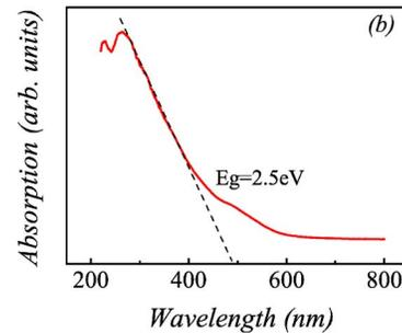
FIG. 3. (a) DSC and TGA curves for the BFO nanowires over  $600\text{--}890^\circ\text{C}$ ; (b) UV-visible diffuse reflectance spectrum of the BFO nanowires.
