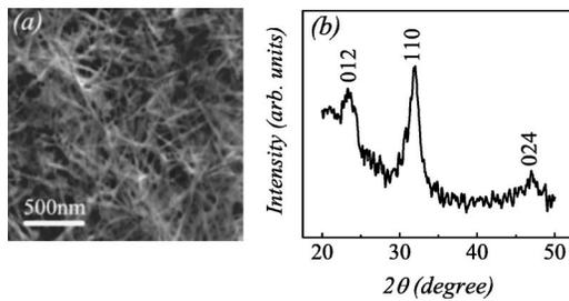
FIG. 1. (a) SEM image and (b) XRD pattern of the BFO nanowires prepared using the sol-gel AAO template method.
