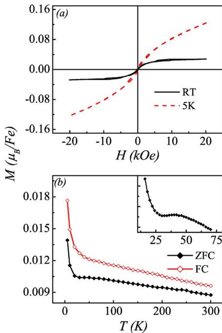
FIG. 4. (a)  $M$ - $H$  hysteresis loops for the BFO nanowires measured at RT and  $T=5$  K. (b)  $M$ - $T$  curves for the BFO nanowires measured under ZFC and FC ( $H=0.1$  T) conditions. The inset presents the ZFC data over a narrower  $T$  range.
