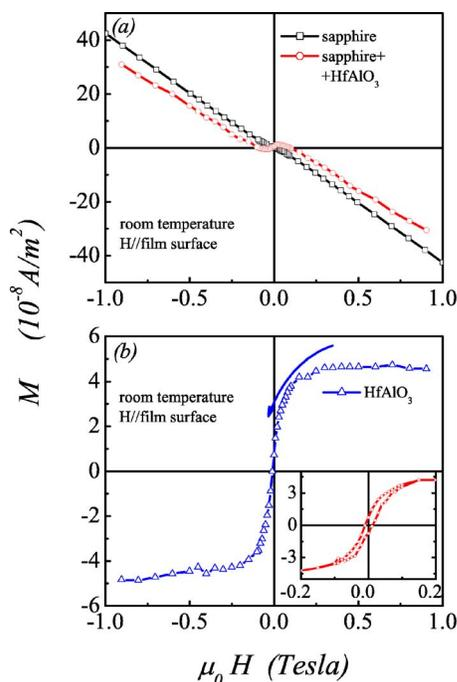
FIG. 2. (Color online) Room-temperature  $M$ - $H$  curves for (a) a bare sapphire substrate and the sapphire substrate plus a 30 nm thick HfAlO<sub>3</sub> film deposited at 600 °C in a vacuum of  $\sim 10^{-5}$  Pa, and for (b) the 30 nm thick HfAlO<sub>x</sub> film after subtracting the diamagnetic background from the sapphire substrate. The inset in (b) is the amplified  $M$ - $H$  hysteresis constructed from the  $M$ - $H$  curve in (b).
