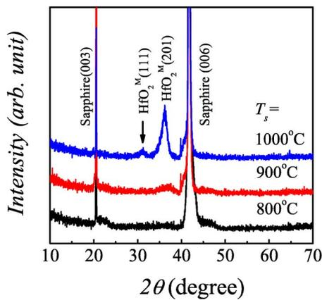
FIG. 1. (Color online) XRD spectra of HfAlO<sub>x</sub> film deposited on (001) sapphire substrates at  $T_s=800^\circ\text{C}$  and rapidly thermally annealed at 900 and 1000 °C for 5 min, respectively.
