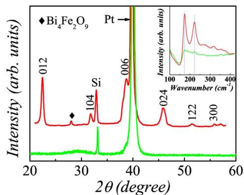
FIG. 1. (Color online) XRD pattern and Raman spectra (inset) of the BFO films prepared by PLD deposited at  $T_s=550$  °C (top line) and 300 °C (bottom line).
