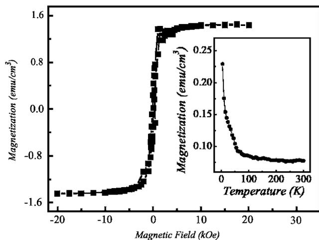
FIG. 3.  $M$ - $H$  hysteresis loop of the amorphous BFO film measured at room temperature. The inset shows the temperature dependent magnetization of the amorphous BFO film.
