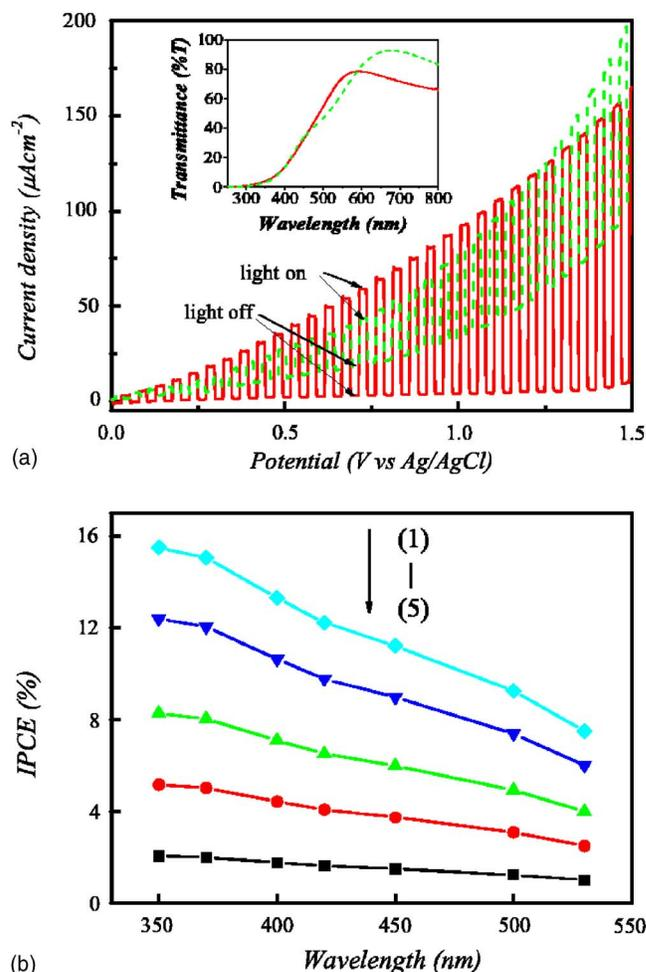
FIG. 2. (Color online) (a) Current-potential dependence of the BFO film electrode under visible-light irradiation. ( $\lambda > 420$  nm, light intensity: 60 mW  $\text{cm}^{-2}$ ). The inset presents optical transmission spectra of BFO films grown on quartz glass. (Solid line for the polycrystalline film and dashed line for the amorphous film.) (b) IPCE of the polycrystalline BFO film electrode measured at different potentials. (1) 1.5 V, (2) 1.2 V, (3) 0.8 V, (4) 0.5 V, and (5) 0.2 V.
