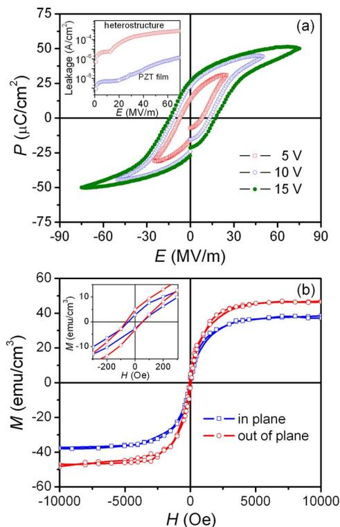
FIG. 2. (Color online) (a) Polarization vs electric field hysteresis ( $P$ - $E$ ) loops for the thin-film heterostructure. Inset is the variation of leakage current density with the applied electric field. (b) The field dependent magnetization ( $M$ - $H$ ) curves for the thin-film heterostructure.
