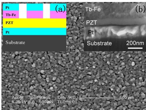
FIG. 1. (Color online) The surface SEM image of the Tb–Fe layer in the thin-film heterostructure. Inset (a) is a sketch of the heterostructure and inset (b) is the fractured cross-sectional SEM image of the heterostructure.
