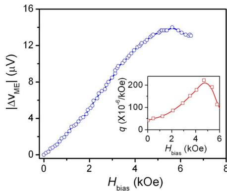
FIG. 3. (Color online) The  $H_{\text{bias}}$  dependence of the induced magnetoelectric voltage increment  $|\Delta V_{\text{ME}}|$  at a given dc magnetic frequency  $f=1.0$  kHz for the thin-film heterostructure. Inset is the  $H_{\text{bias}}$  dependence of piezomagnetic coefficient  $q$  for the pure Tb-Fe nanostructured film prepared by LECBD process.
