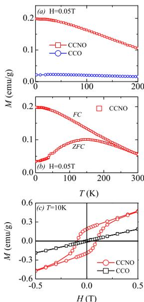
FIG. 2. (Color online) Measured  $M$ - $T$  relation under (a) FC conditions for CCO and CCNO and (b) ZFC and FC conditions for CCNO with a magnetic field of 500 Oe. (c) Measured  $M$ - $H$  hysteresis at 10 K for CCO and CCNO samples, respectively.
