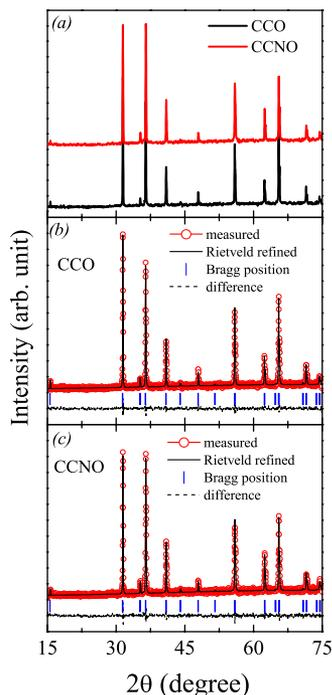
FIG. 1. (Color online) (a) XRD  $\theta$ - $2\theta$  spectra for CCO and CCNO samples (open circle dot, measured, and solid line, using Rietveld structural refinement), respectively. The difference (dashed line, difference) between the measured and Rietveld refined spectra for the two samples, respectively, is plotted with a slight downshift for clarity in (b) and (c). The short vertical solid lines are guides for the eyes for the corresponding Bragg position.
