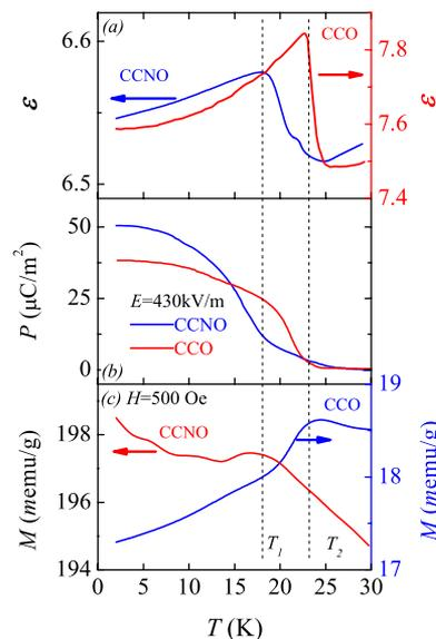
FIG. 3. (Color online) Temperature dependence of (a) dielectric constant  $\epsilon$  and (b) electric polarization  $P$  under  $H=0$  for CCO and CCNO, and magnetization  $M$  for (c) CCO and (d) CCNO.
