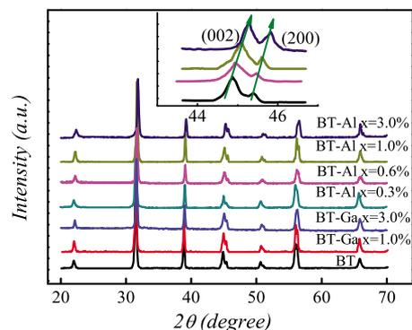
FIG. 1. (Color online) XRD patterns for all the samples. The inset shows the diffraction peaks of (002) and (200) planes for BT-Al at  $x=0$ , 0.6%, 1.0%, and  $x=3.0\%$  from bottom to top, respectively.
