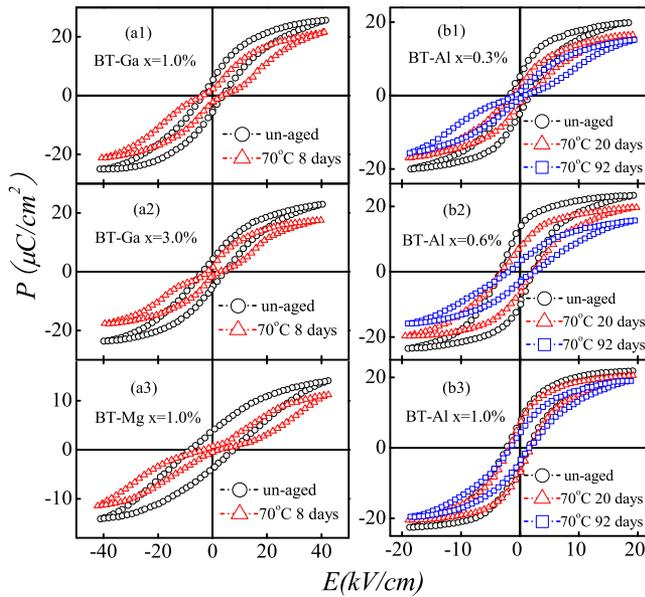
FIG. 2. (Color online) Measured  $P$ - $E$  hysteresis loops at room temperature for several selected samples in the unaged (fresh) state and aged states: (a1) BT-Ga  $x=1.0\%$ , (a2) BT-Ga  $x=3.0\%$ , (a3) BT-Mg  $x=1.0\%$ , (b1) BT-Al  $x=0.3\%$ , (b2) BT-Al  $x=0.6\%$ , and (b3) BT-Al  $x=1.0\%$ . The time (day) and temperature ( $70^\circ\text{C}$ ) for the aging of each sample are labeled, respectively, in each plot.
