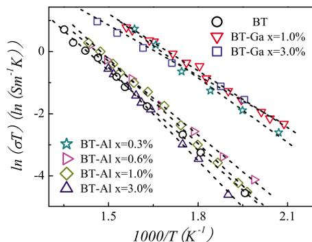
FIG. 3. (Color online) Arrhenius plot  $\ln(\sigma T)$  vs  $1000/T$  for various samples as indicated.
