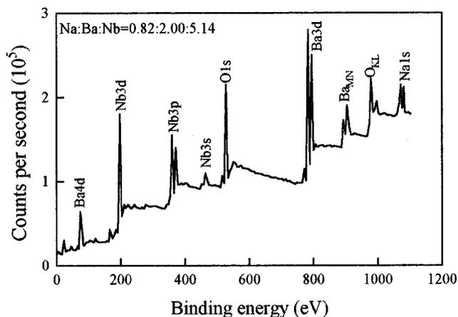
FIG. 4. The XPS spectrum of the as-grown BNN film on (100)-oriented KTP substrate, showing that the atomic ratio of Na:Ba:Nb is 0.82:2.00:5.14.
