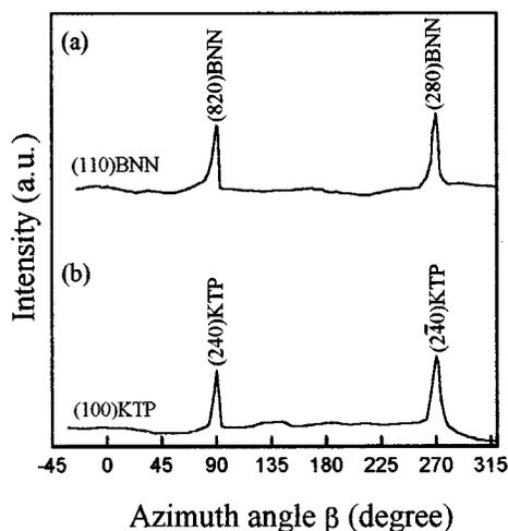
FIG. 2. The x-ray  $\beta$  scan of (a) the (820) and (280) reflections of the (110)-oriented BNN film and (b) the (240) and (240) reflections of the (100)-oriented KTP substrate on which the film was grown.
