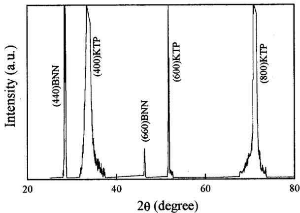
FIG. 1. The x-ray  $\theta$ - $2\theta$  scan of the as-grown BNN film on (100)-oriented KTP substrate.
