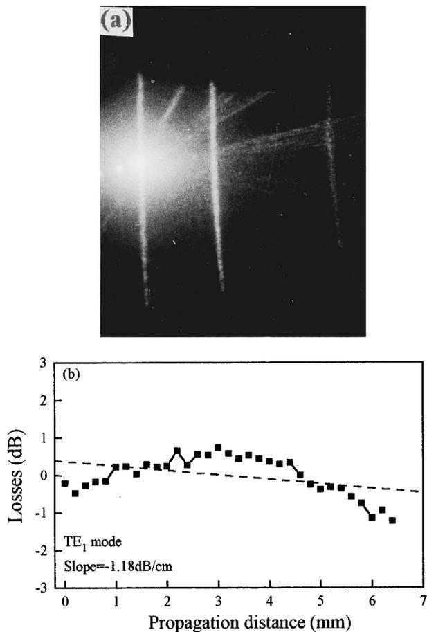
FIG. 5. The observed  $m$  lines of the TE multimodes of a (110)-oriented BNN film grown on (100)-oriented KTP plate (a) and the scattered light intensity out of the TE<sub>1</sub> mode as a function of the propagation distance. (b) The dashed line represents the best-linear fitting.
