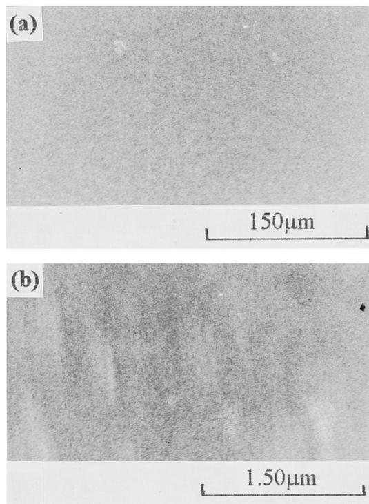
FIG. 3. The SEM pictures showing the surface morphology of the BNN film grown on a (100)-oriented KTP plate.
