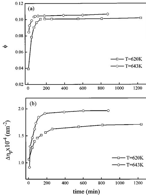
FIG. 3. Time evolution of the volume fraction  $\phi$  of the second supercooled liquid phase (a) and the contrast factor  $\Delta\eta_p$  (b) in the amorphous  $Zr_{41}Ti_{14}Cu_{12.5}Ni_{10}Be_{22.5}$  samples annealed at 620 and 643 K, respectively.
