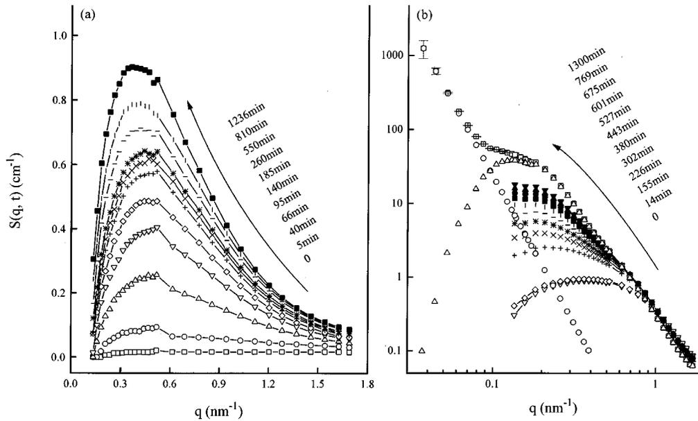
FIG. 1. Time evolution of the scattering spectrum  $S(q, t)$  for the amorphous  $Zr_{41}Ti_{14}Cu_{12.5}Ni_{10}Be_{22.5}$  samples annealed at 620 K for indicated times (a) and subsequently at 673 K for indicated times (b). The solid arrows indicate time flow. In (b), the open square spots represent the scattering at 1300 min, the open circle spots, and up-triangle spots represent  $S_C(q)$  and  $S_D(q)$  at this time.
