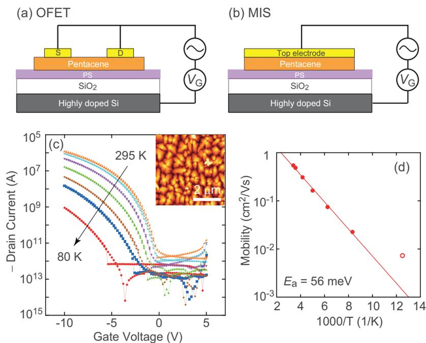
FIG. 1. Schematic structures and measurement configurations of (a) the OFET and (b) the MIS capacitor used in this study. (c) Transfer characteristics of the OFET at a drain voltage of  $-10$  V at various temperatures from 295 to 80 K. The inset shows an atomic force microscope image of the pentacene film. The scale bar corresponds to a  $2 \mu\text{m}$  length. (d)  $\mu_{\text{FET}}$  values of the OFET as a function of the inverse of temperature.
