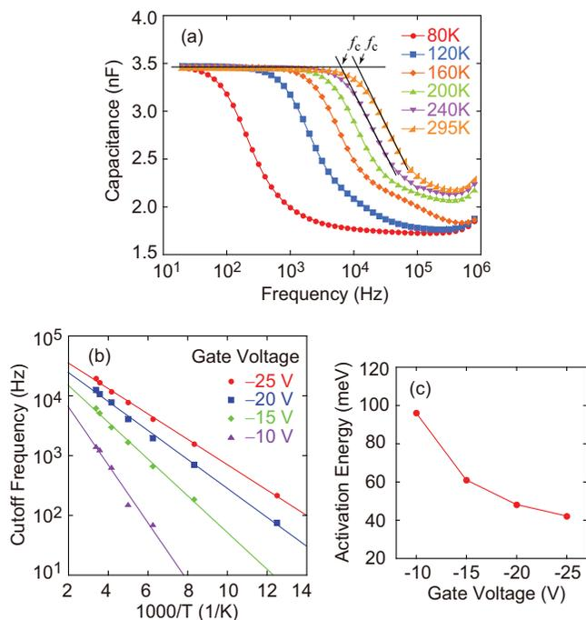
FIG. 4. (a)  $C$ - $f$  characteristics of the OFET at a gate voltage of  $-20$  V at various temperatures. (b) Cutoff frequency of the OFET as a function of the inverse of temperature for various gate voltages. (c) Activation energy of the OFET as a function of gate voltage.
