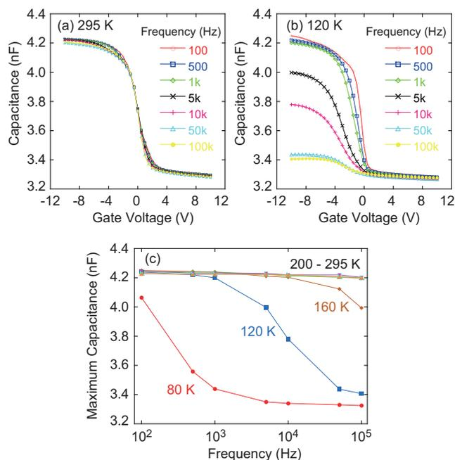
FIG. 2. (a)  $C$ - $V$  characteristics of the MIS capacitor obtained at (a) 295 K and (b) 120 K at various frequencies. (c) The maximum capacitance of the MIS capacitor as a function of frequency for different temperatures.
