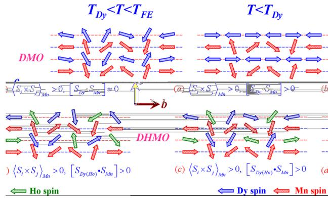
FIG. 1. (Color online) Schematic drawing of the Dy(Ho) and Mn spin configurations at  $T < T_{Dy}$  (right column) and  $T_{Dy} < T < T_{FE}$  (left column) for pure DMO (up row) and DHMO (bottom row). The magnitude and orientation of these spin arrows are drawn only for guide of eyes.
