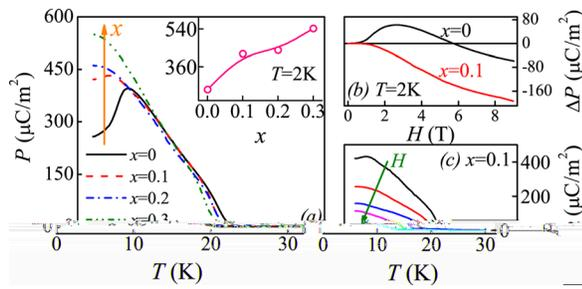
FIG. 4. (Color online) (a) Measured  $P$ - $T$  curves for samples  $x=0, 0.1, 0.2$ , and  $0.3$ , and the inset shows the measured  $P$  at  $T=2$  K as a function of  $x$ , (b) measured  $\Delta P$ - $H$  relations at  $T=2$  K for samples  $x=0$  and  $0.1$ , and (c) measured  $P$ - $T$  curves for various  $H$  (from top to bottom,  $H=0, 3T, 6T$ , and  $9T$ ) for sample  $x=0.1$ .
