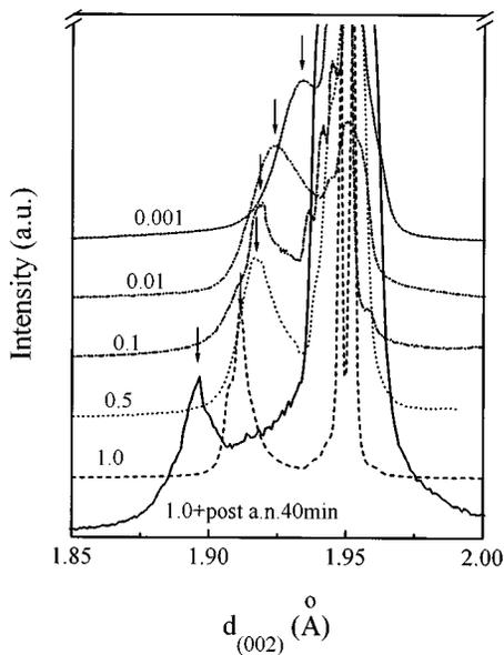
FIG. 1. Local XRD spectra for the LSCO thin films deposited on (001) STO substrates at 650 °C and different  $P_a$  (the values inserted in the figure, unit: mbar). Here “+a.n.40 min” means that the film was postannealed at 1.0 atm  $O_2$  for 40 min, the same below.
