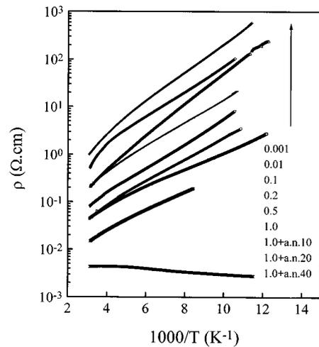
FIG. 2.  $\rho(T)$  for thin film LSCO prepared at different pressures of oxygen. The values of oxygen pressure (mbar) are inserted in the figure.
