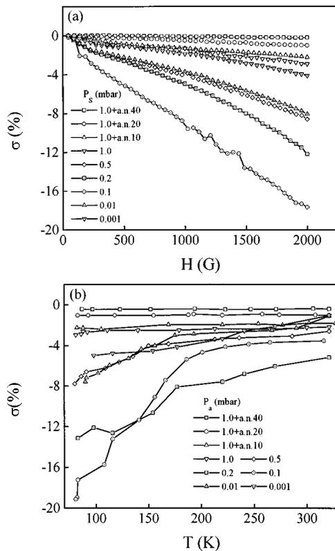
FIG. 4. (a)  $\sigma(H)$  at  $T \approx 85$  K and (b)  $\sigma(T)$  at  $H = 0.2$  T for the thin films prepared at different values of  $P_a$  with and without postannealing. The data represent averaging of four measurements and there appears an error bar of  $\pm(5-10)\%$ .
