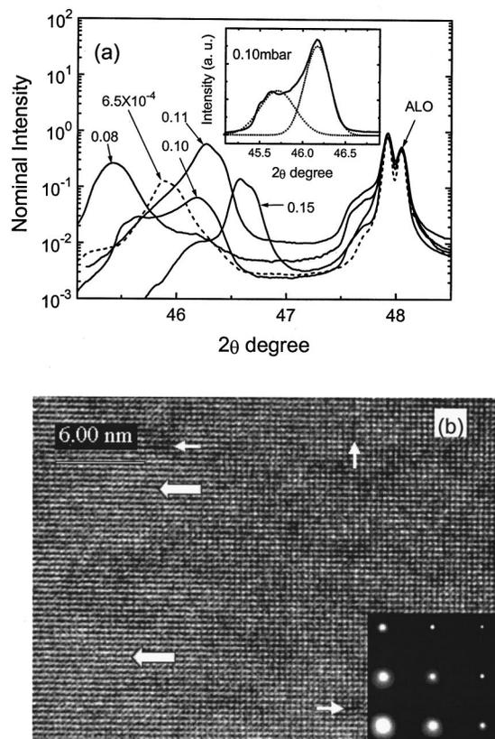
FIG. 3. (a) (002) reflections for films deposited at different  $P_{O_2}$ . Inset is the splitted (002) peak of the 0.10 mbar sample. (b) The planar section high-resolution lattice image for film deposited at  $P_{O_2}=6.5\times 10^{-4}$  mbar. Defects are indicated by white arrows.
