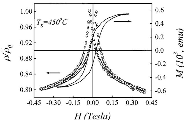
FIG. 2. The  $\rho/\rho_0$ - $H$  and  $M$ - $H$  hysteresis at  $T = 77 \text{ K}$  as a function of time for the LSMO film deposited at  $450^\circ\text{C}$ .
