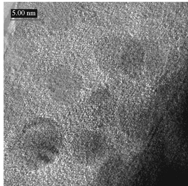
FIG. 3. HRTEM image of the LSMO film deposited at  $450^\circ\text{C}$ .
