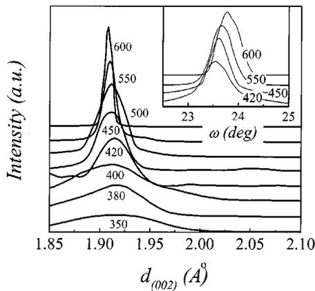
FIG. 1. XRD  $\theta$ - $2\theta$  spectra of the (002) reflection for the LSMO thin films deposited on (001) SrTiO<sub>3</sub> substrates at various temperatures as indicated. The inset gives the  $\omega$  scans with respect to the (002) reflection.
