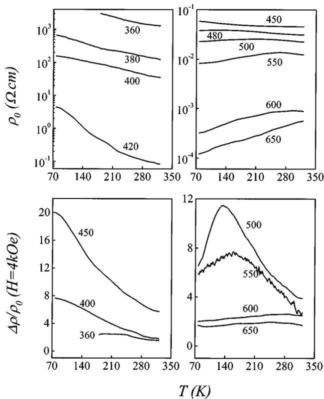
FIG. 5. Zero-field resistivity  $\rho_0$  and magnetoresistance ratio  $\Delta\rho/\rho_0$  at  $H=4$  kOe as functions of temperature for a series of samples deposited at various temperatures as indicated.
