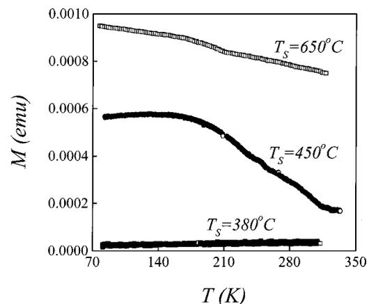
FIG. 4. Magnetization  $M$  at  $H = 8 \text{ kOe}$  as a function of temperature for three samples deposited at 650, 450, and  $380^\circ\text{C}$ , respectively.
